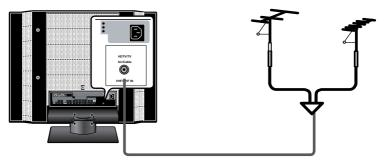
Connect the AC power cord at the back of the TV and connect the power cord to wall outlet.
